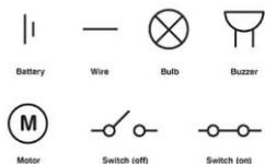
Give children a range of circuit ingredients e.g. a battery, a motor, a bulb and 3 wires. Can they create the circuit and then draw it using the correct recognised symbols?
