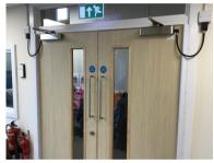
3.4.1.3 Internal doors are generally adequately contrasted against wall surfaces, making the openings easier to identify by a visually impaired person.
