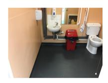
2.6.2.3 The cubicle achieves clear dimensions of 2200mm deep by 2200mm wide which is in excess of current best practice guidelines.
